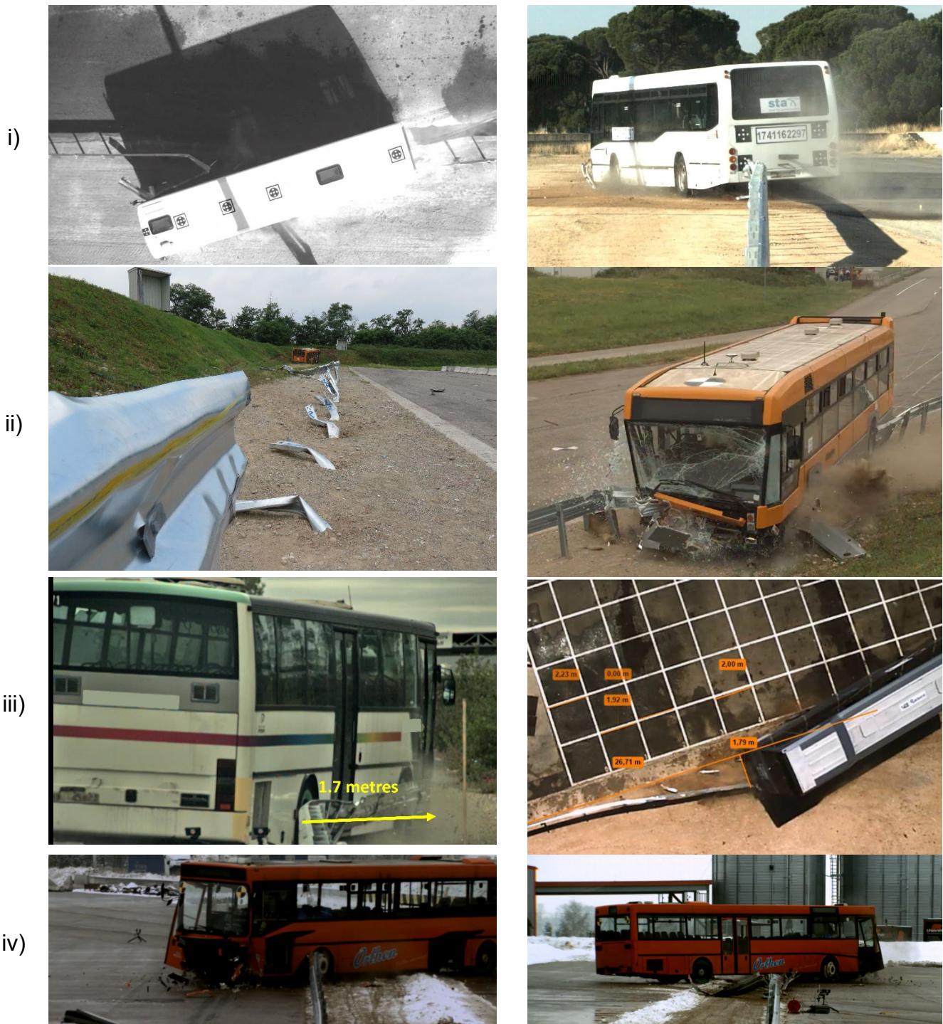
Figure 5 - H2-W4-A crash tests (from top to bottom row): i) 1 st test, vehicle not contained, ii) 2 nd test, vehicle not contained, iii) 3 rd test, system exceeds working width by 2 classes, iv) 4 th test, vehicle not contained
