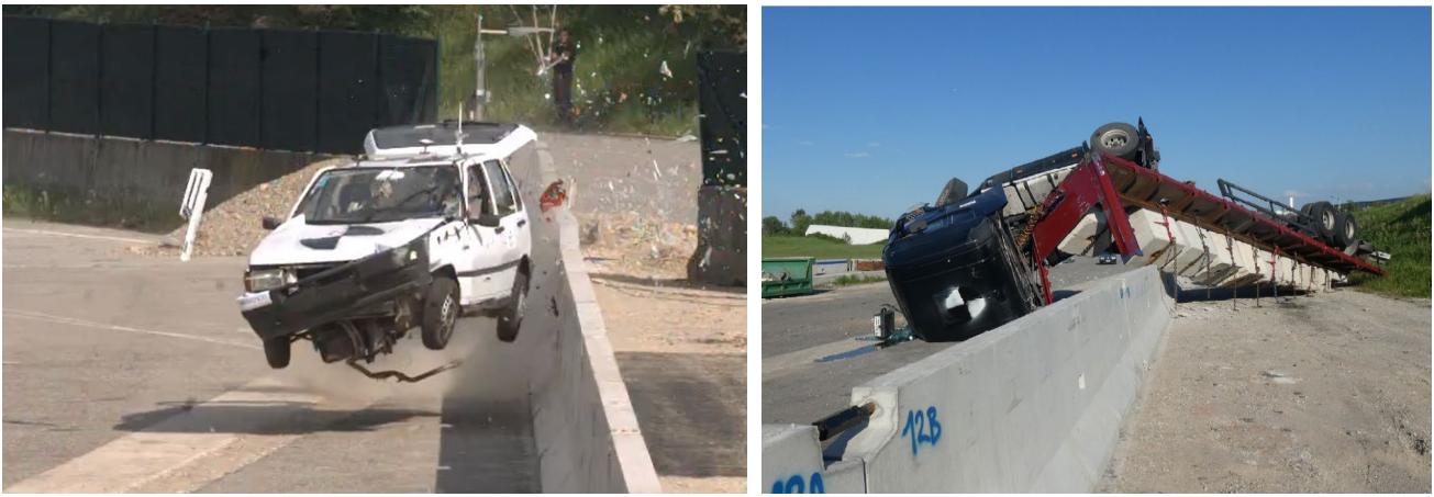
Figure 7 - TB11 crash test result ASI value 1.53 (left), TB81 crash test result with rolled over crash vehicle (right)
