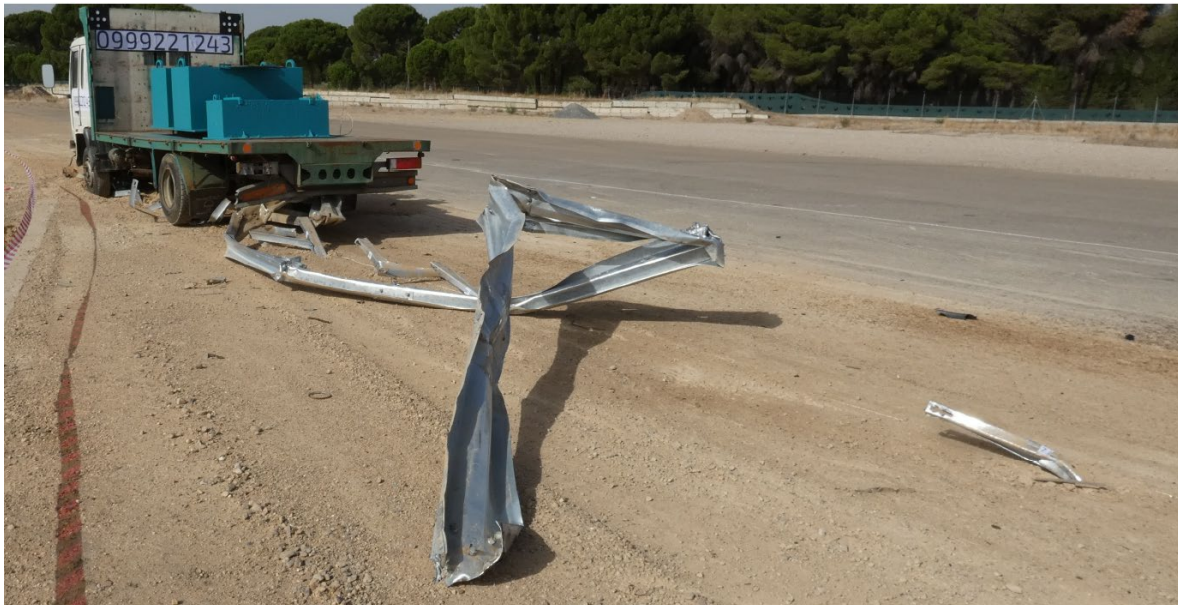
Figure 8 - TB42 sketch of impact area (top), result of crash test with deformed barrier (bottom)
