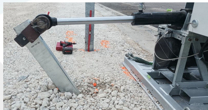
Laboratory test – soil/post resistance assessment
