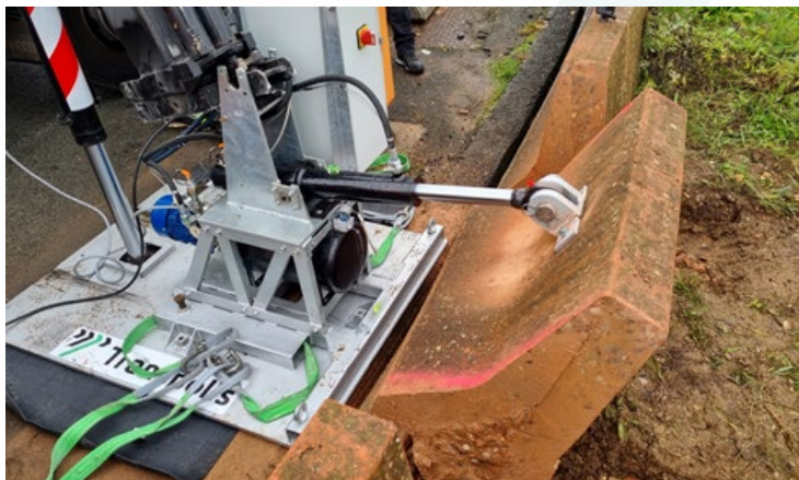
Field test on a highway concrete barrier
